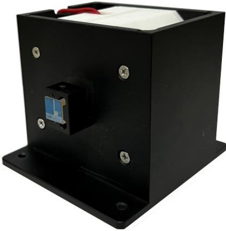
Fig. 3 Photograph of the FADOF. The housing of the PBS is made of aluminum. The PBS is fixed to the front and back of the FADOF and is used to select the laser with a specific polarization. The cesium vapor cell is wrapped with a heating wire for temperature control and placed in a Teflon insulation layer with a tight fit between them for better insulation. The Teflon layer is placed in an aluminum housing and secured with screws. The cesium vapor cell is made of glass, with a length of 3 cm and a diameter of 1.5 cm, and is filled with 10 torr Ar as buffer gas. The Teflon insulation layer has holes to place
